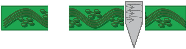
3. A thin (about  $3\mu\text{m}$ ) seeder layer is formed on both sides and inside the via by electroless copper plating.
