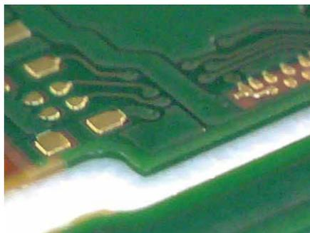
**Aiming to reduce the dust by covering the board edge by Solder Resist.**
