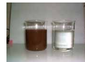
(左:原液・右:濃縮装置濾過後水) (Left side : Waste Water-Right : After filtration)
